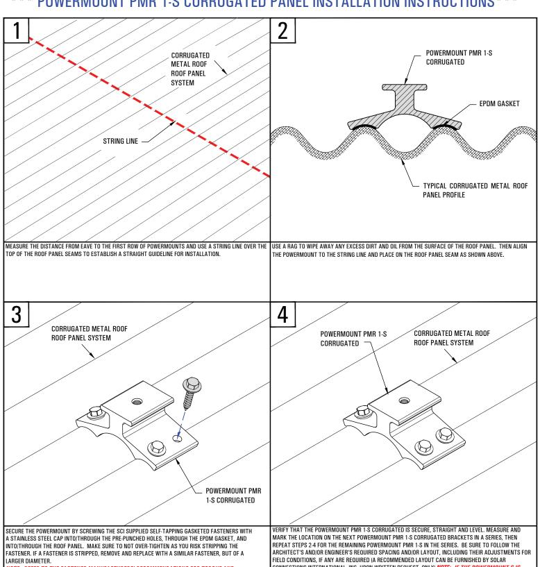
NOTE: REFER TO THE FASTENER MANUFACTURERS' RECOMMENDATIONS FOR TORQUE AND WASHER SEATING REQUIREMENTS REFORE INSTALLATION.
