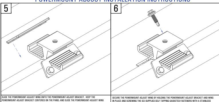
SLIDE THE POWERMOUNT-ADJUST WING ONTO THE POWERMOUNT-ADJUST BRACKET. KEEP THE POWERMOUNT-ADJUST BRACKET CENTERED ON THE PANEL AND SLIDE THE POWERMOUNT-ADJUST WING ALL THE WAY DOWN. MAKE SURE THE POWERMOUNT-ADJUST WING IS AS FAR OVER AND DOWN AS POSSIBLE AND FIRMLY PRESS THE POWERMOUNT-ADJUST WING AGAINST THE PANEL MAKING CONSISTENT CONNECTION BETWEEN THE EPDM GASKET AND THE PANEL ITSELF, PRIOR TO FASTENING.
