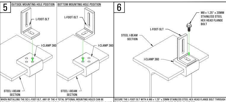
UTILIZED, USING AN ORIENTATION ENSURING THAT THE L-FOOT-SLT IS INSTALLED ON TOP OF THE I-CLAMP 360. SO THAT THE ENTIRE L-FOOT-SLT BRACKET BASE IS SITTING DIRECTLY ON THE TOP FACE OF THE
