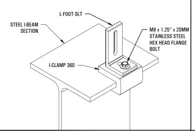
VERIFY THAT THE L-FOOT-SLT IS SECURE STRAIGHT AND LEVEL. REPEAT STEPS 5 AND 6 FOR THE REMAINING L-FOOT-SLT'S TO BE INSTALLED ON TOP OF THE I-CLAMP 360'S IN THE SERIES. BE SURE TO FOLLOW THE ARCHITECT'S AND/OR ENGINEER'S REQUIRED SPACING AND/OR LAYOUT, INCLUDING THEIR ADJUSTMENTS FOR FIELD CONDITIONS, IF ANY ARE REQUIRED (A RECOMMENDED LAYOUT CAN BE FURNISHED BY SOLAR CONNECTIONS INTERNATIONAL, INC. UPON WRITTEN REQUEST, ONLY).
