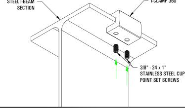
VERIFY THAT THE I-CLAMP 360 IS SECURE, STRAIGHT AND LEVEL. MEASURE AND MARK THE LOCATION OF THE NEXT I-CLAMP 360'S LOCATION, THEN REPEAT STEPS 2-4 FOR THE REMAINING I-CLAMP 360'S IN THE
