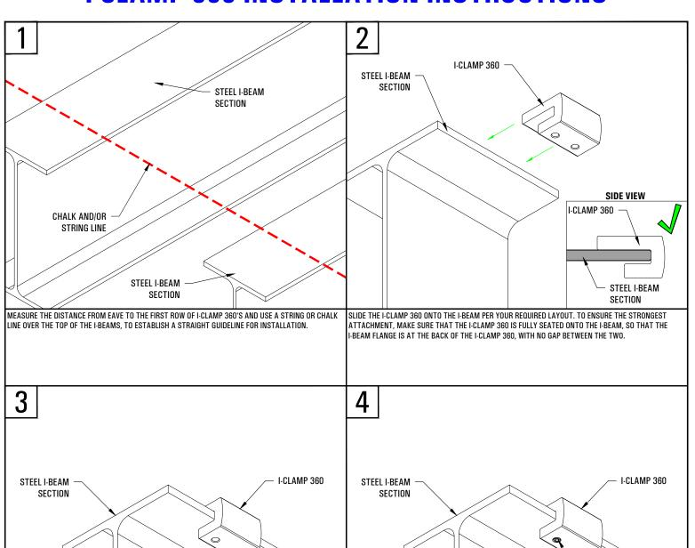
3/8" - 24 x 1" STAINLESS STEEL CUP POINT SET SCREWS SECURE THE I-CLAMP 360 WITH THE TWO 3/8" - 24 x 1" STAINLESS STEEL CUP POINT SET SCREWS (OR THE OPTION B BEING: M8 x 1.25 x 20MM STAINLESS STEEL HEX HEAD FLANGE BOLT) TO THE STEEL I-BEAM ON
