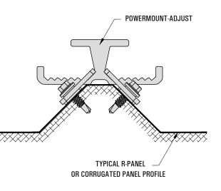
POSSIBLE AND FIRMLY PRESS THE POWERMOUNT-ADJUST WING AGAINST THE PANEL MAKING CONSISTENT
