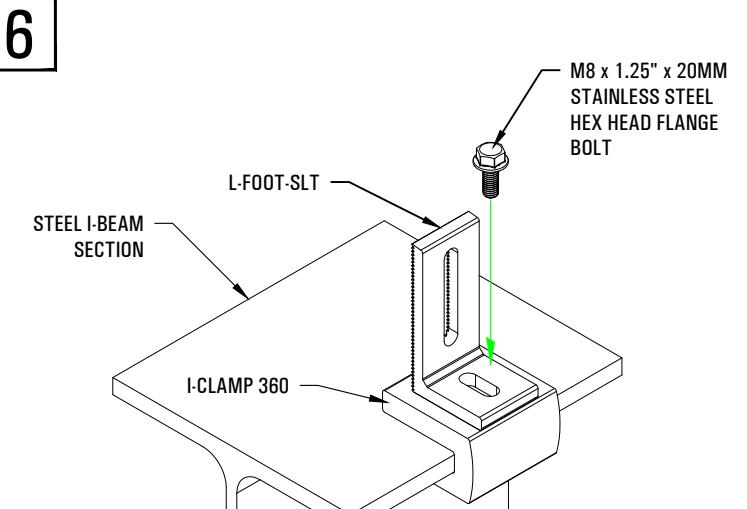
WHEN INSTALLING THE SCI L-FOOT-SLT, ANY OF THE 4 TOTAL OPTIONAL MOUNTING HOLES CAN BE UTILIZED, USING AN ORIENTATION ENSURING THAT THE L-FOOT-SLT IS INSTALLED ON TOP OF THE I-CLAMP 360, SO THAT THE ENTIRE L-FOOT-SLT BRACKET BASE IS SITTING DIRECTLY ON THE TOP FACE OF THE I-CLAMP 360 ITSELF.
