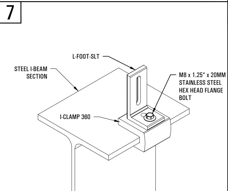
VERIFY THAT THE L-FOOT-SLT IS SECURE STRAIGHT AND LEVEL. REPEAT STEPS 5 AND 6 FOR THE REMAINING L-FOOT-SLT'S TO BE INSTALLED ON TOP OF THE I-CLAMP 360'S IN THE SERIES. BE SURE TO FOLLOW THE ARCHITECT'S AND/OR ENGINEER'S REQUIRED SPACING AND/OR LAYOUT, INCLUDING THEIR ADJUSTMENTS FOR FIELD CONDITIONS, IF ANY ARE REQUIRED (A RECOMMENDED LAYOUT CAN BE FURNISHED BY SOLAR CONNECTIONS INTERNATIONAL, INC. UPON WRITTEN REQUEST, ONLY).
