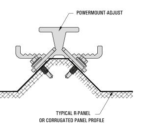
POSSIBLE AND FIRMLY PRESS THE POWERMOUNT-ADJUST WING AGAINST THE PANEL MAKING CONSISTENT
