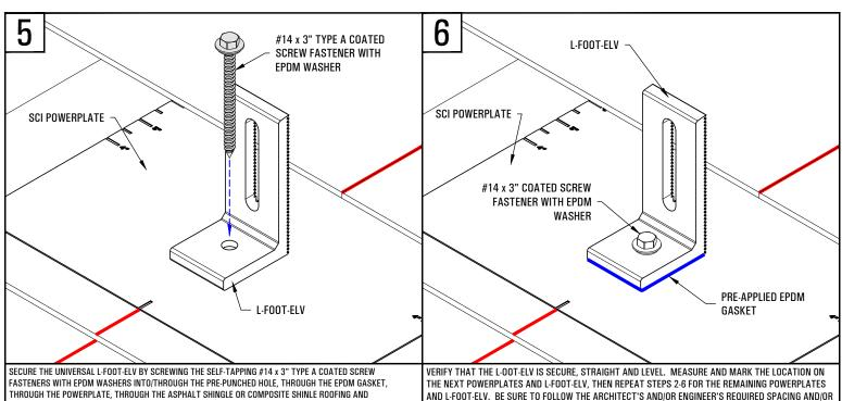
UNDERLAYMENT, THROUGH THE ROOF DECK AND INTO THE WOOD FRAMING MEMBERS BELOW. MAKE SURE TO NOT OVER-TIGHTEN AS YOU RISK STRIPPING THE FASTENER. IF A FASTENER IS STRIPPED, REMOVE AND REPLACE WITH A SIMILAR FASTENER, BUT OF A LARGER DIAMETER.
