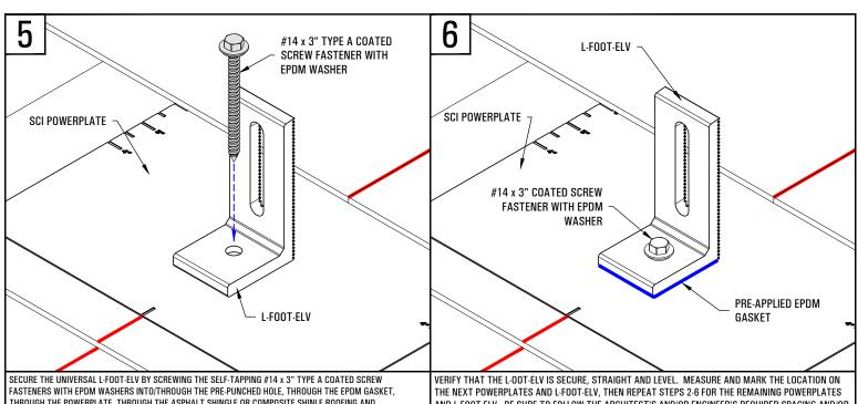
THROUGH THE POWERPLATE. THROUGH THE ASPHALT SHINGLE OR COMPOSITE SHINLE ROOFING AND UNDERLAYMENT, THROUGH THE ROOF DECK AND INTO THE WOOD FRAMING MEMBERS BELOW. MAKE SURE TO NOT OVER-TIGHTEN AS YOU RISK STRIPPING THE FASTENER. IF A FASTENER IS STRIPPED, REMOVE AND REPLACE WITH A SIMILAR FASTENER, BUT OF A LARGER DIAMETER. REFER TO THE FASTENER MANUFACTURERS' RECOMMENDATIONS FOR TOROUF AND WASHER SEATING
