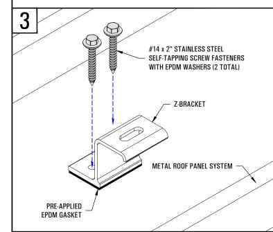
**Z-BRACKET** PRE-APPLIED **EPDM GASKET** METAL ROOF PANEL SYSTEM
