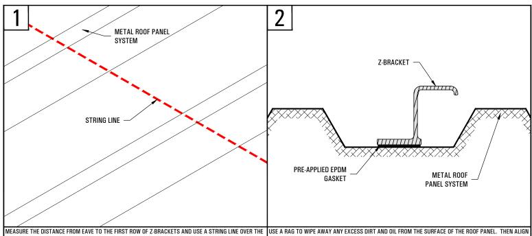
TOP OF THE ROOF PANEL CORRUGATIONS TO ESTABLISH A STRAIGHT GUIDELINE FOR INSTALLATION.
